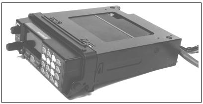
Figure 30 - Handle Assembly In LOCKED Position
